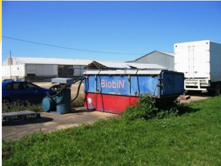
Photograph 10. The Biobin© Sealed Composting Unit used on Farm C
