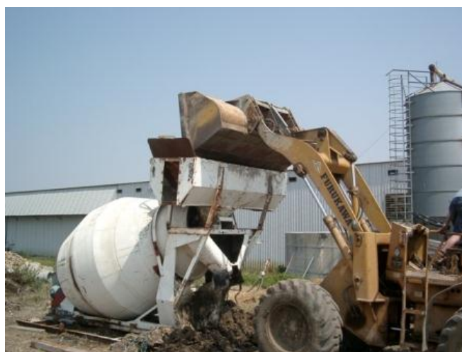
Photograph 11. Rotary Composter Built from Cement Mixing Barrel
