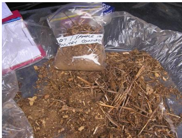
Photograph 14. Sample from Farm F showing large particle size of the carbon material
