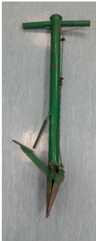
Figure 27. Left – PottiPutki planter in action. Middle – planter with beak mechanism in closed position ready for inserting into soil. Right – beak mechanism open ready for planting. The seedling is dropped down the hollow tube section of the planter and then the planter lifted up out of the way. Soil around the seedling is compacted by the operator’s feet.
