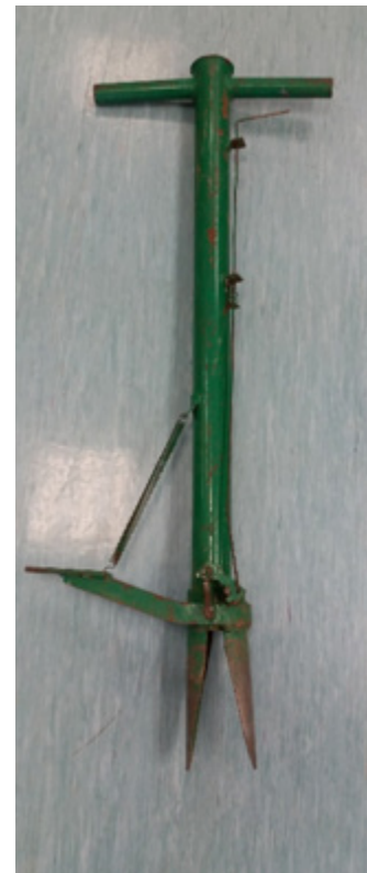
Figure 27. Left – PottiPutki planter in action. Middle – planter with beak mechanism in closed position ready for inserting into soil. Right – beak mechanism open ready for planting. The seedling is dropped down the hollow tube section of the planter and then the planter lifted up out of the way. Soil around the seedling is compacted by the operator’s feet.
